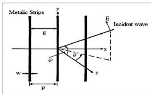
Figure 3: Plane wave incidence upon an inductive Strip grating. For a capacitive strip grating, replace the incident electric field (E) with a magnetic field (H)
