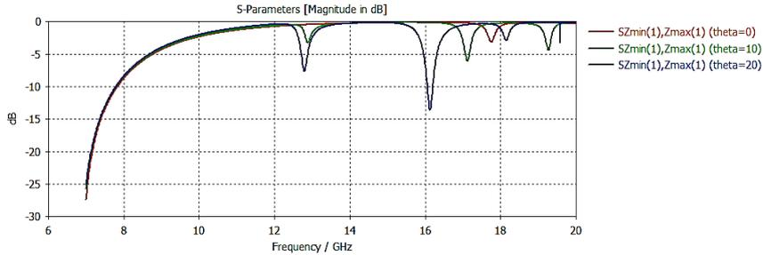
Figure.9. Incidence angle variation of pass band unit cell in TE mode
