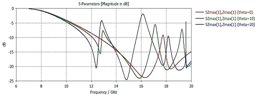
Figure.7. Incidence angle variation of stop band unit cell in TE
