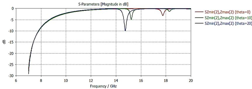
Figure.10 Incidence angle variation of pass band unit cell in TM mode
