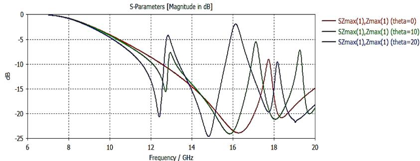
Figure 8. Incidence angle variation of stop band unit cell in TM
