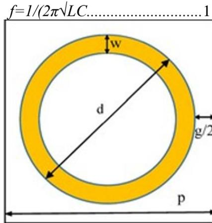
Figure 1: The geometry circular loop FSS
