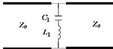
Figure 2: LC circuit
